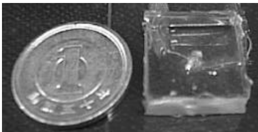
Fig. 10: Sensing and powering coils in silicon rubber.
