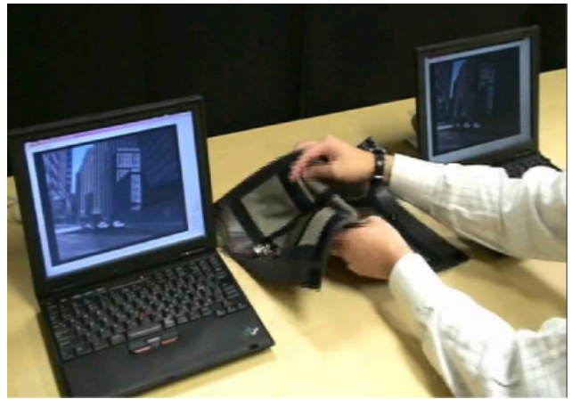
Fig. 11 A scene of the experiment. The cell bridges are mounted on stretchable conductive fabrics. Stretching didn’t affect the communication.
