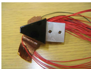
Fig. 12. One of the eight linear arrays. The surface is covered with a water-proof film. 40 pieces of PZT transducers are included in a linear array.
