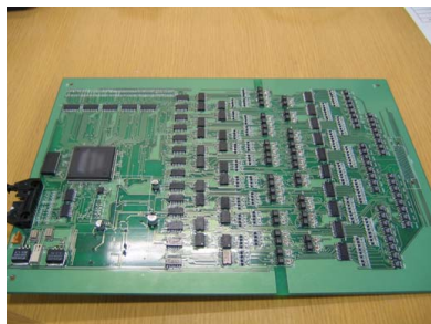
Fig. 11. Photograph of the driving circuit board. A driving circuit board includes a CPLD, a memory, and 40 channel amplifiers. Eight driving circuit boards are used for driving 320 PZT transducers.
