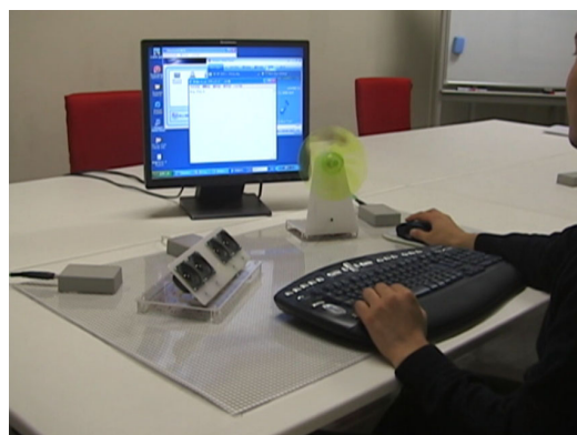
Fig. 4: A loudspeaker, mouse, keyboard, and fan without wires or batteries.
