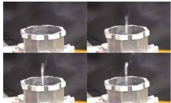
Fig. 2 A jet of water created by the prototype tactile display.
