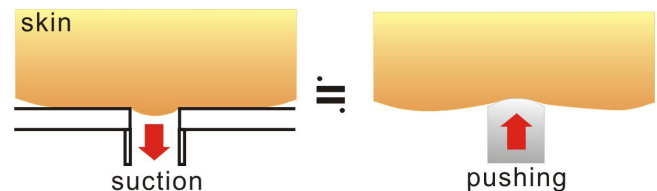
Figure 2. Schematic illustration of suction pressure stimulation. Drawing air causes a sensation as if something is pushing up.
